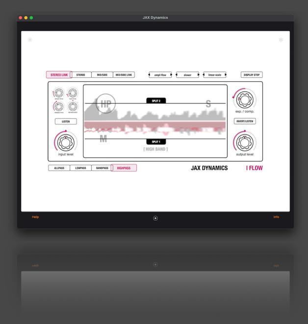
The JAX Dynamics PRO is a set of really easy to use visual audio units for altering the levels of sound in time dependency. The signal flow and important action of the internal DSP is displayed in realtime, unleashing the secrets of operation, even easy to understand for a novice.
